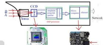
**Gambar 2.8** Diagram Alur CCTV Network<sup>[2]</sup>
