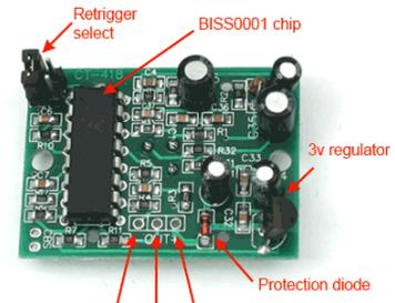
Gambar 2.18 Blok Sistem PIR Sensor<sup>[10]</sup>
