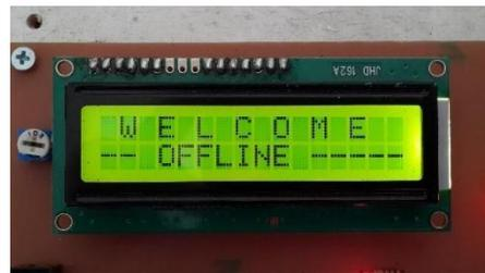
Gambar 2.6 LCD 16 x 2
