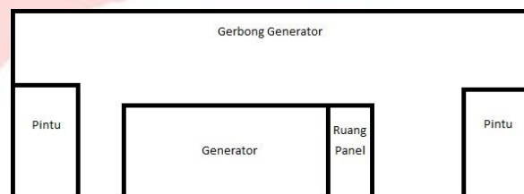
Gambar 4.3 Denah Gerbong Generator
