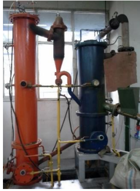
Gambar 1. Reaktor Gasifikasi Circulating Fluidized Bed
