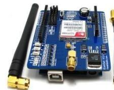
Gambar 3 GSM Arduino Shield
