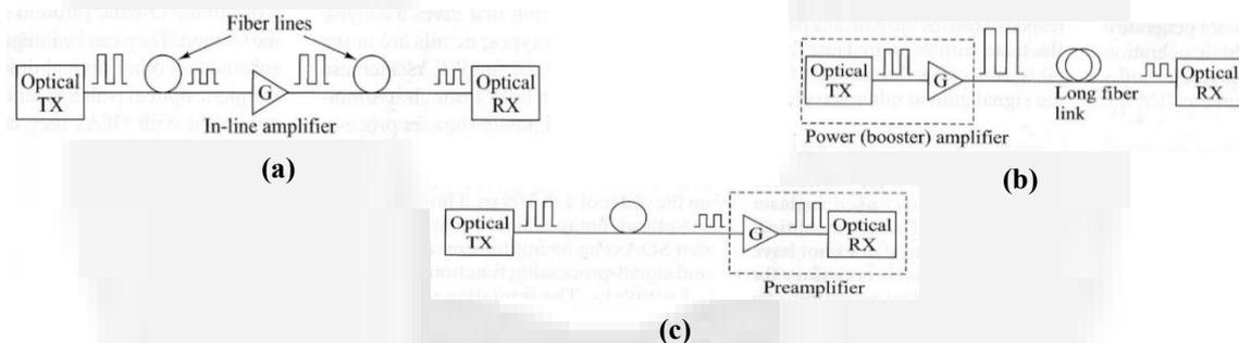
Gambar 1 Penggunaan *optical amplifier* (a) *In-line amplifier* (b) *Booster amplifier* (c) *Pre-amplifier* [6]
