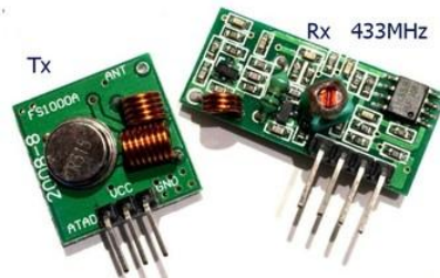
Gambar 4. Transmitter RF433MHz(kiri) dan receiver RF433MHz(Kanan)
