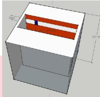
**Gambar 1 Sensor Kapasitif**
