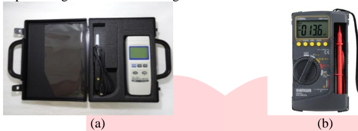
Gambar 3. 2 Alat ukur (a) Magnetic Meter Model MG-3002, (b) Multimeter
