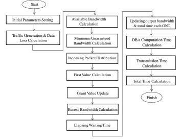
Figure 3. Flowchart multi partition DBA
