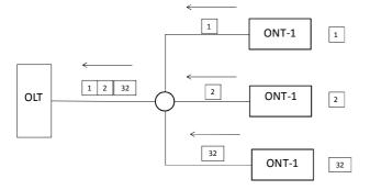
Figure 1. Upstream communication principle of GPON
