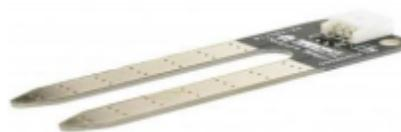
Gambar 2.3 Soil Moisture Sensor
