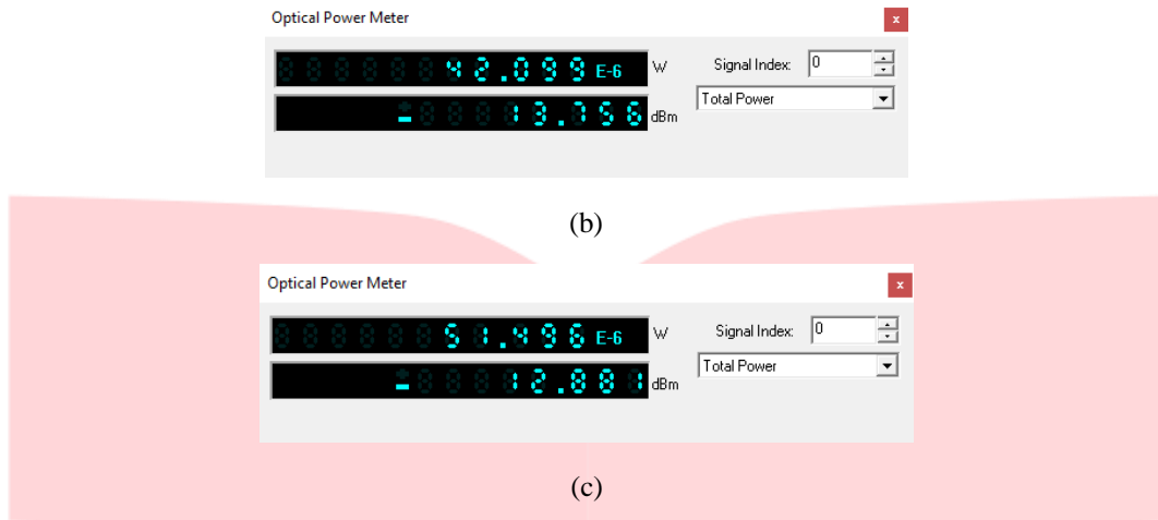
Gambar 4.4 Hasil power received terburuk tiap kecamatan (a) Kec. Loksado (b) Kec. Kandangan (c) Kec. Kalumpang sisi downstream
