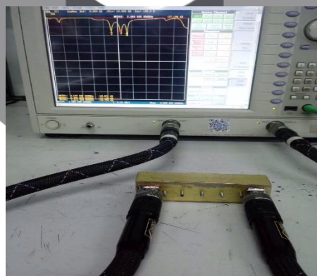
Gambar 6. Realisasi Bandpass Filter Compline Cavity
