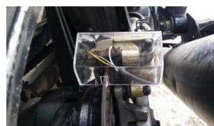
Gambar 4.2 Casing pelindung sensor tampak belakang.
