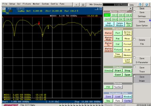
Gambar 11 nilai return loss pengukuran
