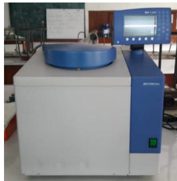
Gambar 0.1 Kalorimeter Bom IKA C2000 Basic.
