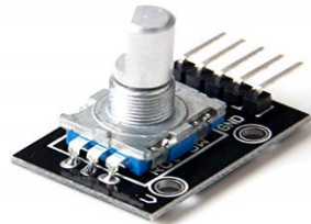
Gambar 1 . Digital Rotary encoder KY-040
