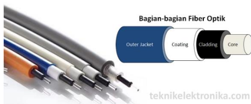
Gambar 1 Bagian-bagian fiber optik [7]
