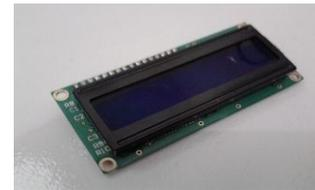
Gambar 3. LCD 2x16
