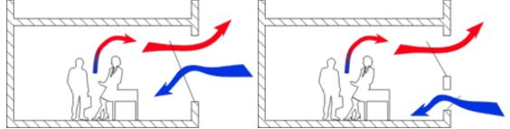
**Figure 1.** Single sided and single double sided ventilation Source: www.dyerenvironmental.co.uk/natural\_vent\_systems.html
