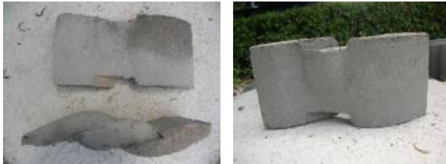
Figure 4. The wind translucent concrete blocks (gedheg brick) (Source: Gunawan et al, 2014)
