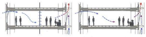
Figure 2. Cross ventilation system with and without partition Source: GSW-energy-ventilation.htm
