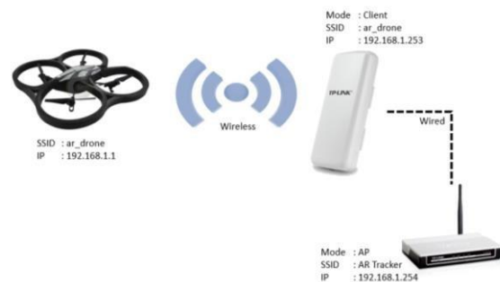
Gambar 14 Topologi Wifi Extender
