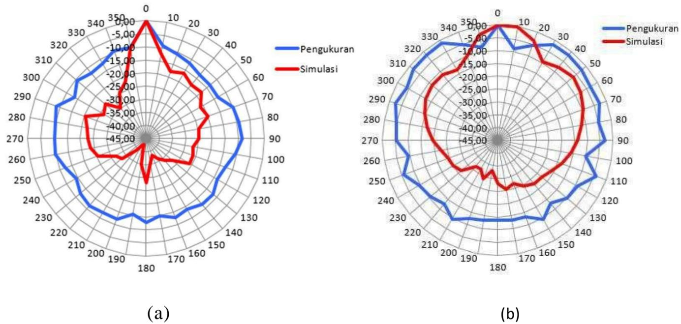
Gambar 9 Hasil Pengukuran Polaradiasi (a) Azimuth (b) Elevasi
