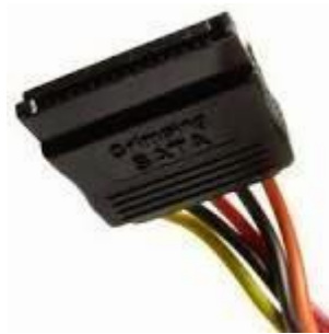
Gambar 2.1.4 SATA Power Connector
