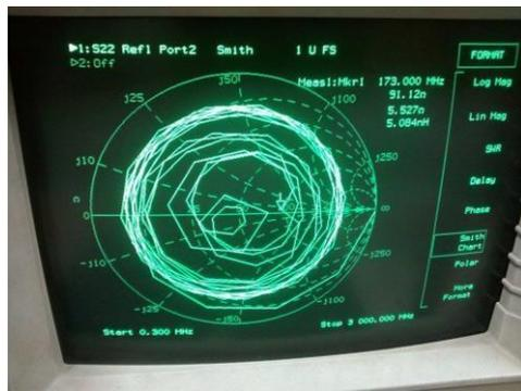
GAMBAR 4 6 (HASIL PENGUKURAN IMPEDANSI ANTENA TX)
