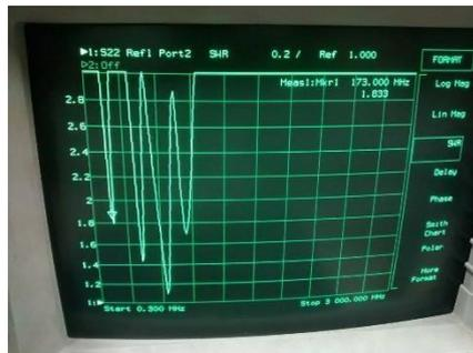
GAMBAR 4 5 (HASIL PENGUKURAN VSWR ANTENA TX)
