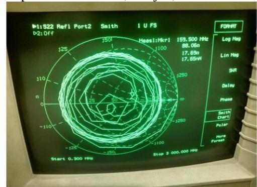
GAMBAR 4 1 (HASIL PENGUKURAN IMPEDANSI ANTENA RX)
