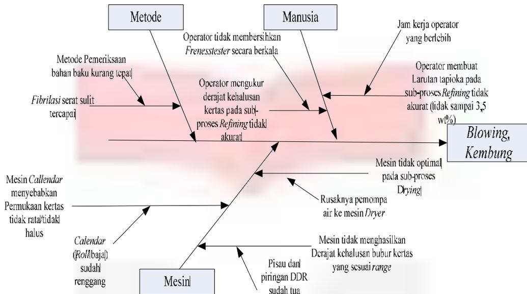
Gambar 9. Fishbone diagram cacat Bonding Kembang
