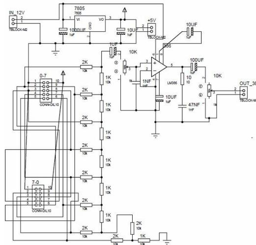
Figure 4 Schematic of the modulator
