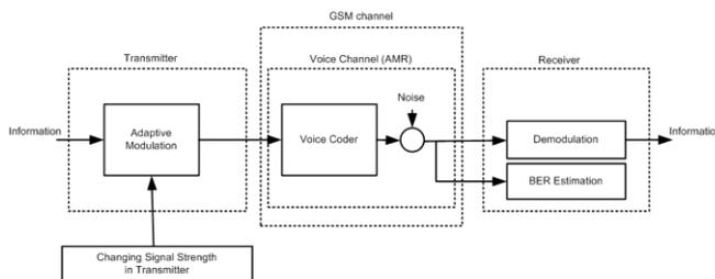
Figure 3 Proposed adaptive modulation without feedback channel
