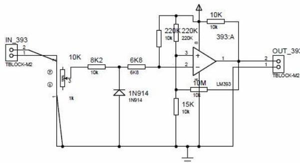
Figure 5 Schematic of the demodulator
