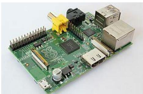
Gambar 1. Tampilan Board Raspberry Pi tipe B
