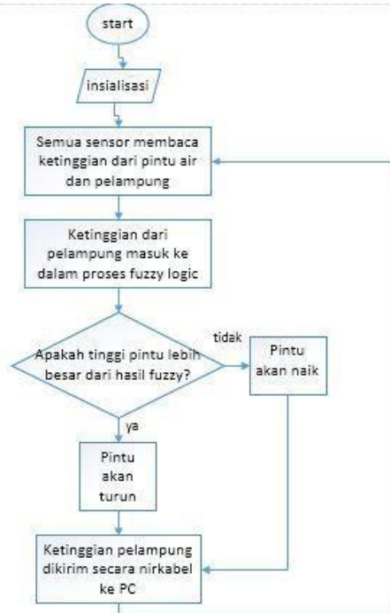
Gambar 2 flow chart sistem
