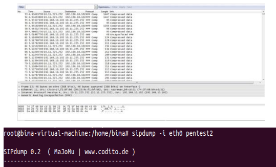
Fig 5. Sniffing VoIP communication without VPN solutions
