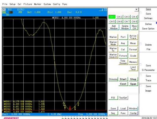
Gambar 4.1 (a) Hasil pengukuran VSWR di Network Analyzer
