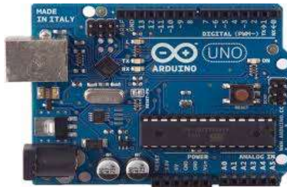
Gambar 2.5 Board Mikrokontroler Arduino UNO [7]
