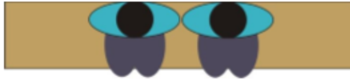
Figure 10. Position of people sit at center and the side distance 75cm. Bench Dimension 210 x 60 cm
