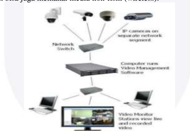
Gambar 2.2 Arsitektur IP-based Camera
