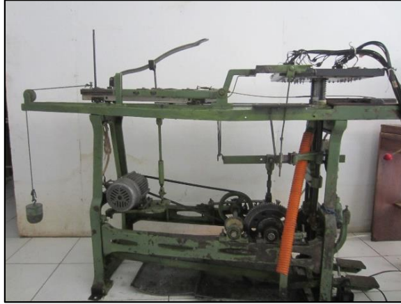
Figure I.2 Punching Machine Existing (PT. BIG, 2016)
