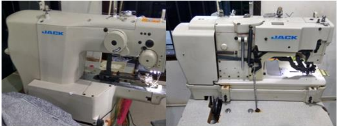
Figure IV.8. Mesin Button Installation
