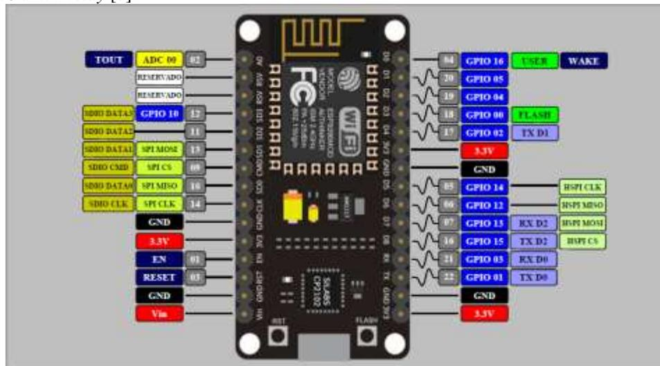
Gambar 2. 2 Datasheet NodeMCU
