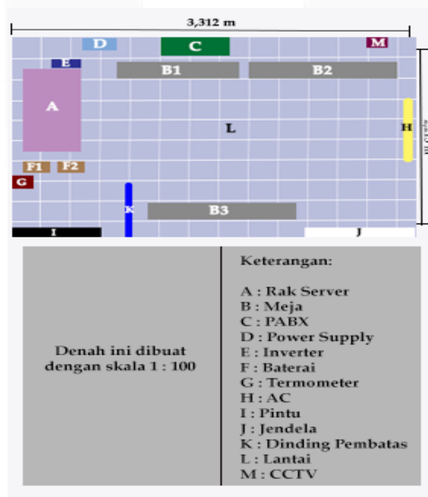
Gambar 3. Layout Ruang Data Center RSIM Sumberrejo
