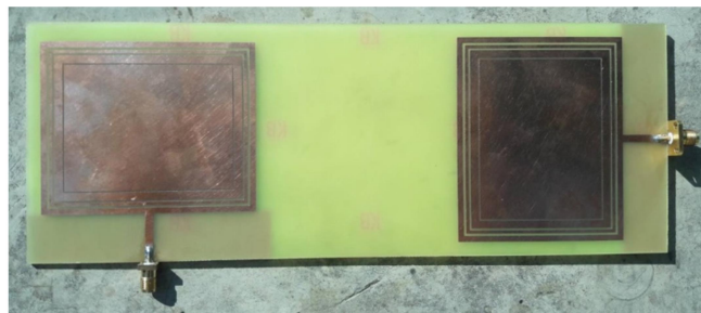
Gambar 2.5 Realisasi antenna MIMO 2x2 dual band
