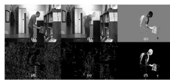
Gambar 9. Dataset office . (a) Input , (b) Background modeling , (c) Foreground detection , (d) Pesebaran fitur , (e) Persebaran fitur , (f) Background subtraction
