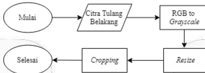
Gambar 5 Diagram alir pre-processing
