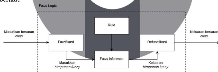
Gambar 5. Proses Fuzzy Logic Controller
