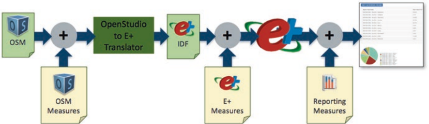
Fig. 6.15 High level OpenStudio workflow with Measures
