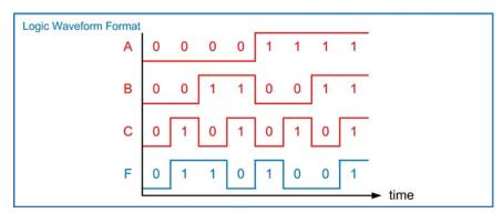
Fig. 3.4 Example logic waveform
