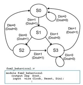
**Fig. 9.2** FSM 2 state diagram and module definition
