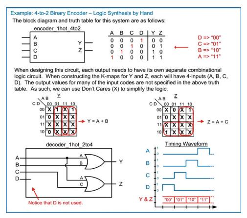
**Example 6.8** 4-to-2 binary encoder: logic synthesis by hand
