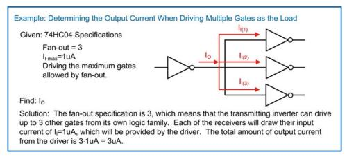
**Example 3.4**Determining the output current when driving multiple gates as the load
