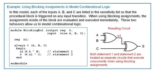
**Example 8.1**Using blocking assignments to model combinational logic
