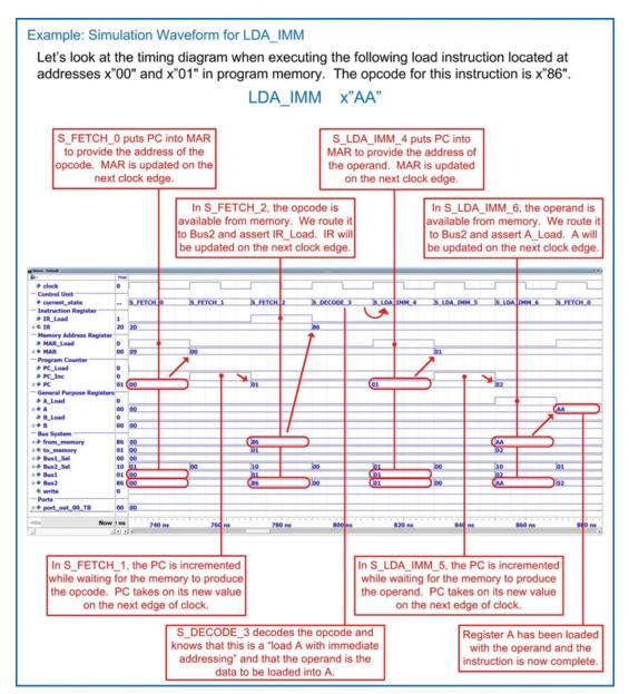
**Example 13.13**Simulation waveform for LDA\_IMM
