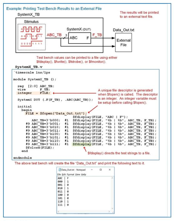
**Example 8.14**Printing test bench results to an external file
