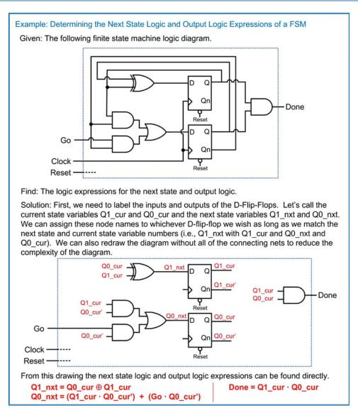
**Example 7.28**Determining the next state logic and output logic expression of a FSM
