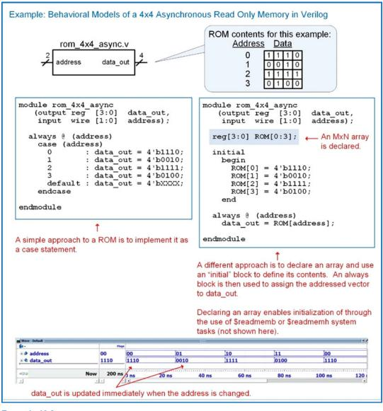
**Example 10.2**Behavioral models of a 4×4 asynchronous read-only memory in Verilog
