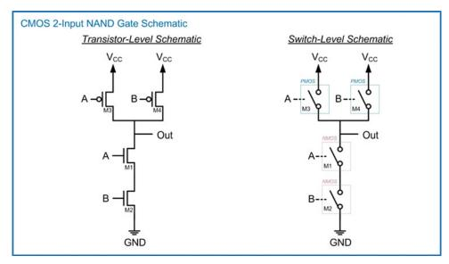
Fig. 3.24 CMOS 2-input NAND gate schematic
