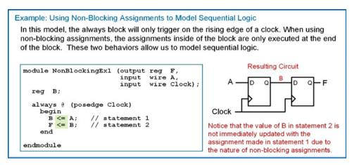
**Example 8.2**Using non-blocking assignments to model sequential logic
