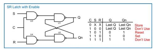
Fig. 7.12 SR Latch with enable schematic
