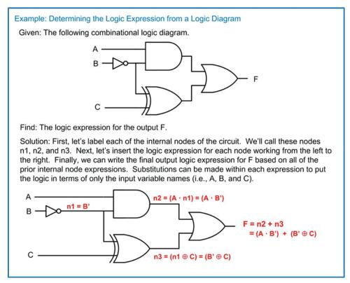
**Example 4.12**Determining the logic expression from a logic diagram
