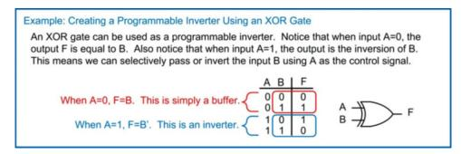
**Example 12.16**Creating a programmable inverter using an XOR gate
