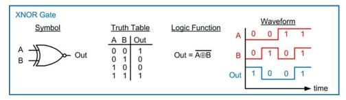
**Fig. 3.13** 2-input XNOR gate symbol, truth table, logic function, and logic waveform
