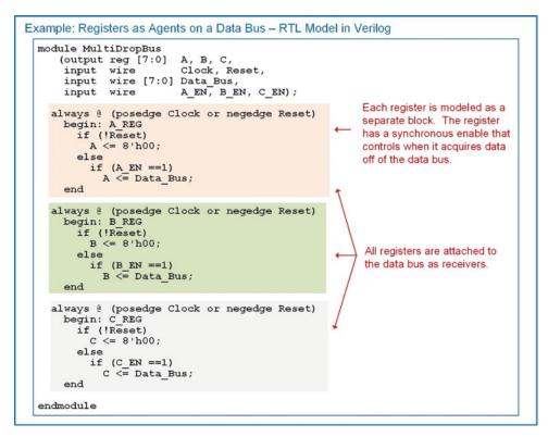
**Example 9.26**Registers as agents on a data bus: RTL model in verilog
