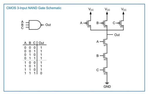
Fig. 3.26 CMOS 3-input NAND gate schematic
