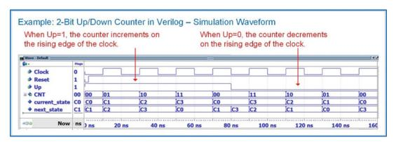
**Example 9.19**2-bit up/down counter in verilog: simulation waveform
