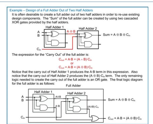
**Example 12.3** Design of a full adder out of half adders
