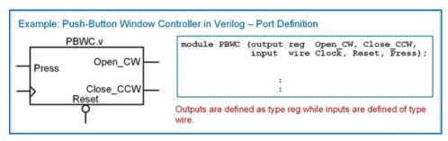
**Example 9.7**Push-button window controller in verilog: port definition
