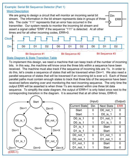
**Example 7.9**Serial bit sequence detector (part 1)
