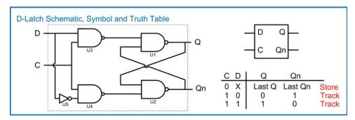
**Fig. 7.14** D-Latch schematic, symbol, and truth table
