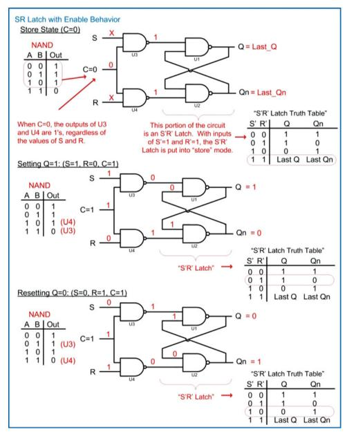
Fig. 7.13 SR Latch with enable behavior: store, set, and reset
