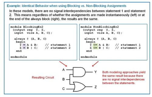
**Example 8.3** Identical behavior when using blocking vs. non-blocking assignments
