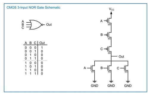
Fig. 3.29 CMOS 3-input NOR gate schematic
