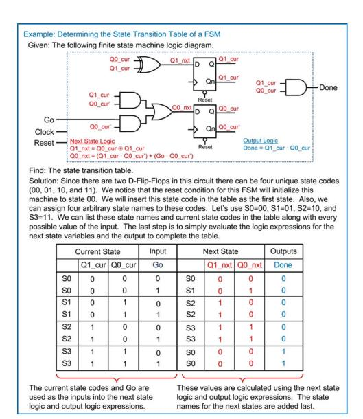
**Example 7.29**Determining the state transition table of a FSM
