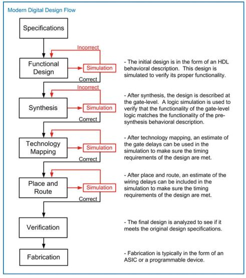
Fig. 5.7 Modern digital design flow
