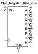
**Fig. 9.11** 16-bit shift register block diagram
