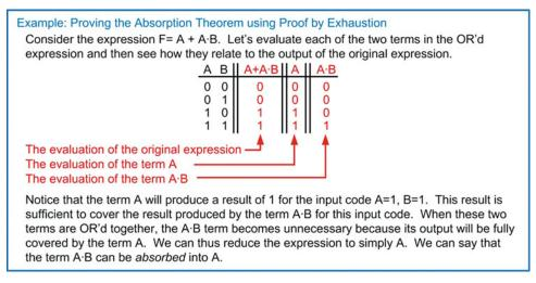
**Example 4.6**Proving the absorption theorem using proof by exhaustion
