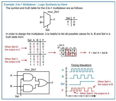
**Example 6.10** 2-to-1 multiplexer: logic synthesis by hand
