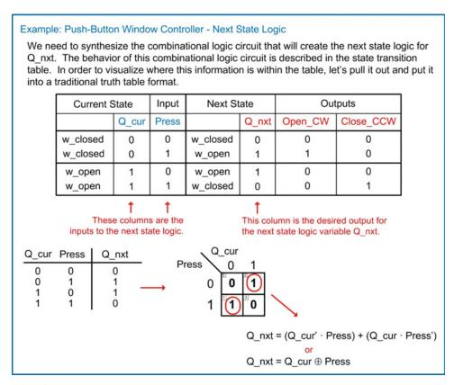
**Example 7.6**Push-button window controller: next state logic
