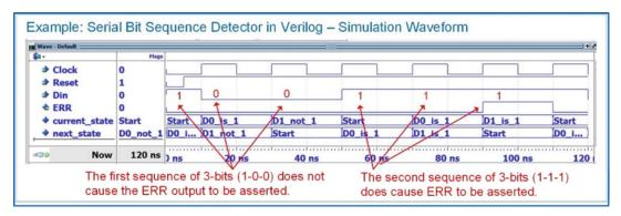
**Example 9.13**Serial bit sequence detector in verilog: simulation waveform
