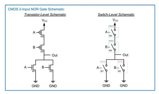
Fig. 3.27 CMOS 2-input NOR gate schematic
