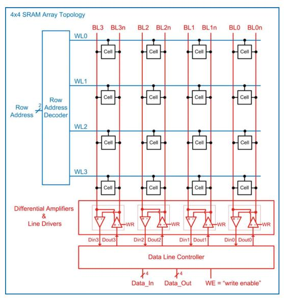
**Fig. 10.11** 4×4 SRAM array topology
