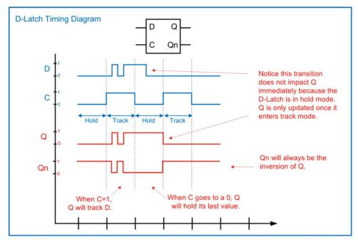
Fig. 7.15 D-Latch timing diagram
