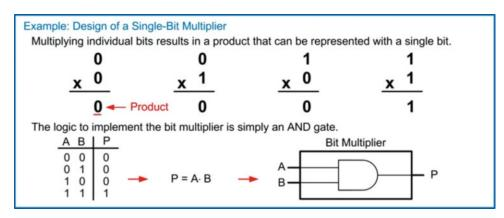
**Example 12.20**Design of a single-bit multiplier
