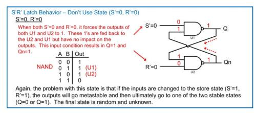
Fig. 7.10 S'R' Latch behavior: don't use state (S' = 0 and R' = 0)
