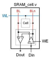
Fig. 10.20 SRAM cell block diagram
