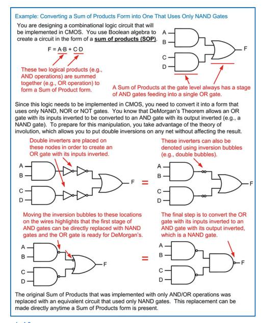
**Example 4.8**Converting a sum of products form into one that uses only NAND gates
