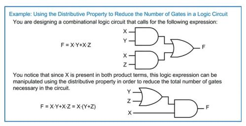
**Example 4.5**Using the distributive property to reduce the number of logic gates in a circuit
