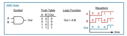
**Fig. 3.7** 2-input AND gate symbol, truth table, logic function, and logic waveform
