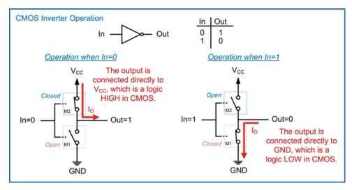
Fig. 3.23 CMOS inverter operation
