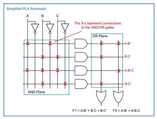
Fig. 11.2 Simplified PLA schematic
