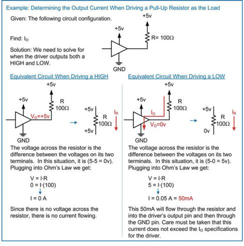
**Example 3.5**Determining the output current when driving a pull-up resistor as the load
