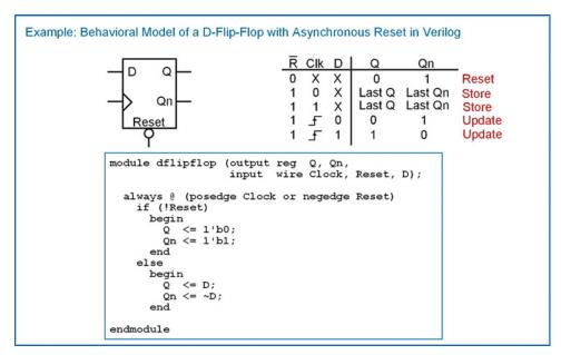
**Example 9.3**Behavioral model of a D-flip-flop with asynchronous reset in verilog
