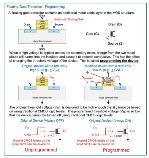
Fig. 10.7 Floating-gate transistor – Programming
