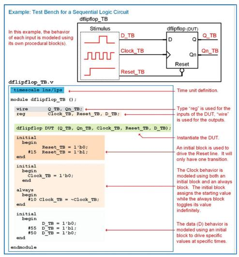
**Example 8.10**Test bench for a sequential logic circuit
