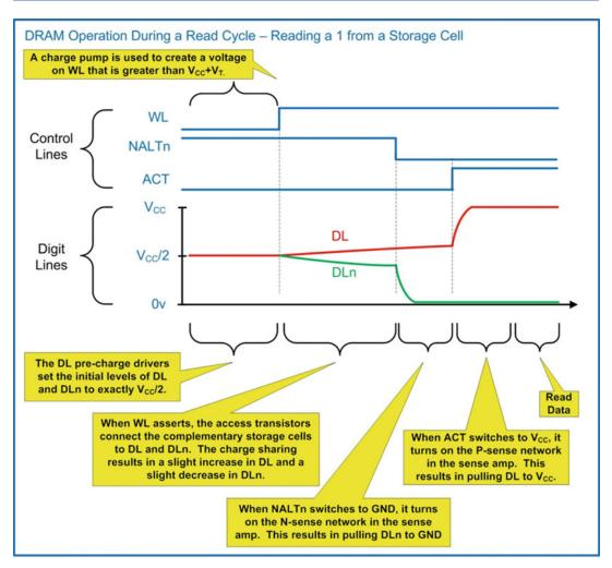
**Fig. 10.19**DRAM operation during a read cycle – Reading a 1 from a storage cell
