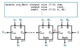
**Fig. 12.4** 4-bit RCA module definition
