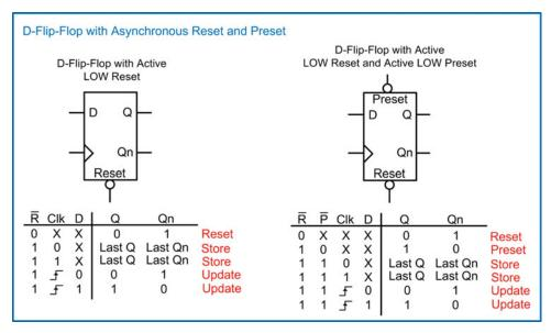
**Fig. 7.18**D-flip-flop with asynchronous reset and preset
