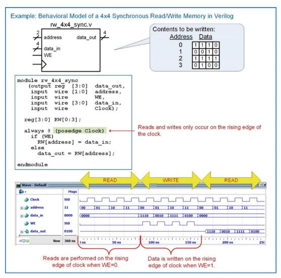
**Example 10.5**Behavioral model of a 4×4 synchronous read/write memory in Verilog
