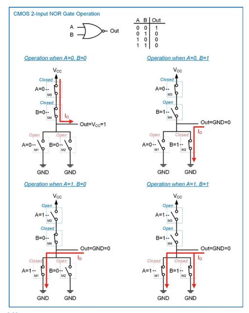
Fig. 3.28 CMOS 2-input NOR gate operation
