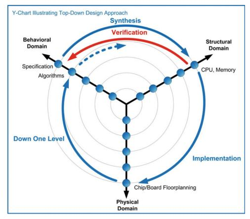
**Fig. 5.4** Y-chart illustrating top-down design approach
