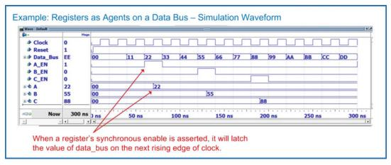
**Example 9.27**Registers as agents on a data bus: simulation waveform
