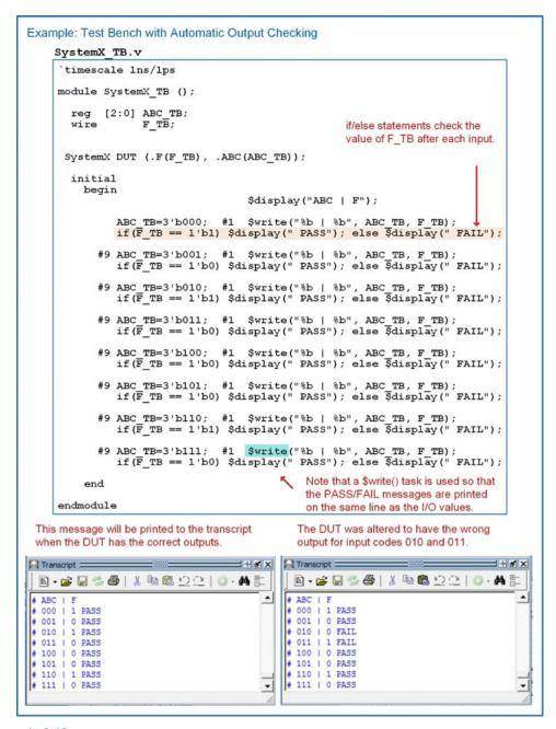
**Example 8.12**Test bench with automatic output checking
