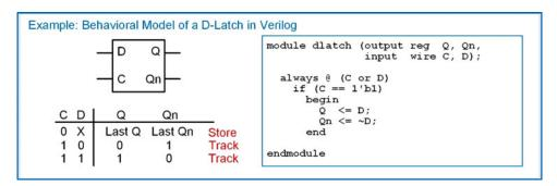
**Example 9.1**Behavioral model of a D-latch in verilog
