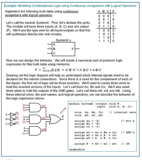
Example 5.2 Modeling combinational logic using continuous assignment with logical operators
