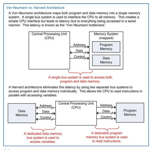
Fig. 13.5 Von Neumann vs. Harvard architecture
