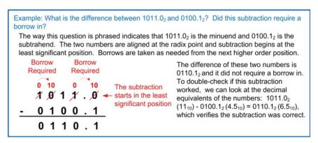
**Example 2.17**Multiple-bit binary subtraction
