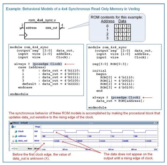
**Example 10.3** Behavioral models of a 4×4 synchronous read-only memory in Verilog
