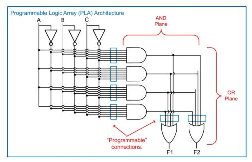
**Fig. 11.1** Programmable logic array (PLA) architecture
