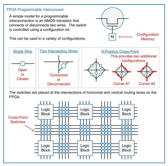
**Fig. 11.11** FPGA programmable interconnect
