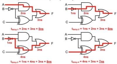
The longest delay path through this circuit is from B to F in which the signal traverses the inverter, XOR gate, and OR gate ( $t_{delay-3}$ ). This path takes 8ns to compute. Since we must always consider the longest delay path when calculating how fast this circuit can operate, we can say that the delay of this combinational logic circuit is <u>8ns</u>.
