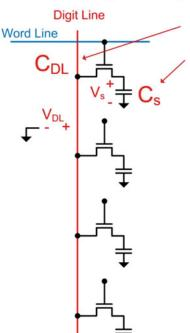
To illustrate how charge sharing limits the voltage that is developed on the digit line, let's consider a simple example where the cell is storing a logic 1 ( $V_S$ =+3.3v) and the digit line is initially set to  $V_{DL}$ =1.65v. The capacitance of the storage cell is  $C_S$ =10 pF while the capacitance of the digit line is  $C_{DL}$ =150 pF. We want to solve for the voltage on the digit line <u>after</u> the access transistor is closed.
