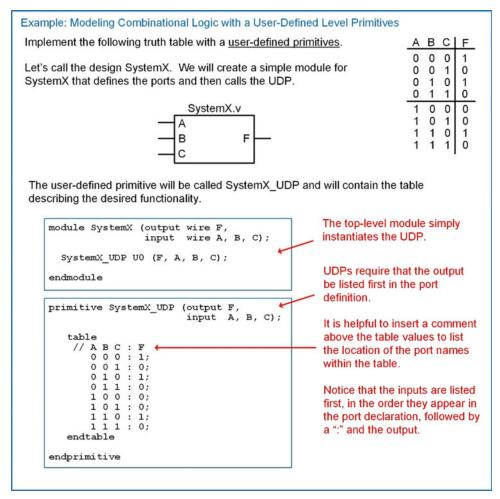
**Example 5.10**Modeling combinational logic circuits with a user-defined primitive
