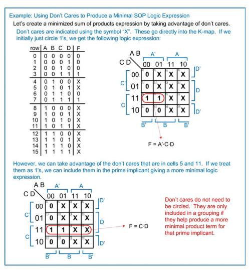
**Example 4.30**Using don't cares to produce a minimal SOP logic expression
