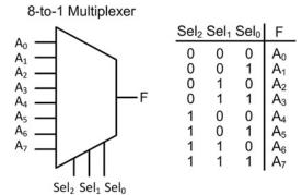
**Fig. 6.7** 8-to-1 multiplexer functionality
