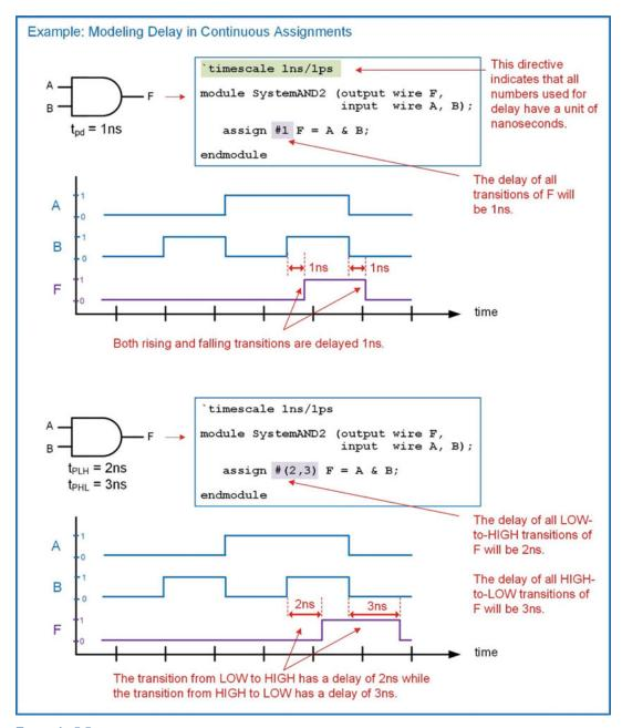
**Example 5.5** Modeling delay in continuous assignments
