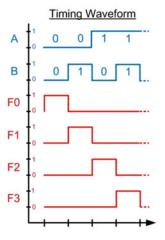
Example 6.1 2-to-4 one-hot decoder: logic synthesis by hand
