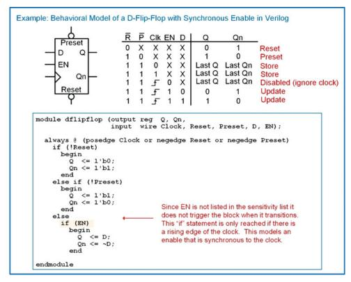
**Example 9.5**Behavioral model of a D-flip-flop with synchronous enable in verilog
