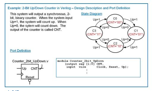
**Example 9.17**2-bit up/down counter in verilog: design description and port definition
