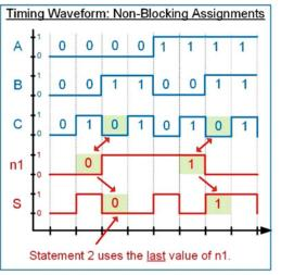
**Example 8.4**Different behavior when using blocking vs. non-blocking assignments (1)
