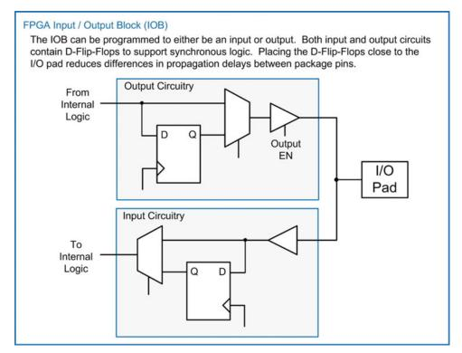
Fig. 11.12 FPGA input/output block (IOB)
