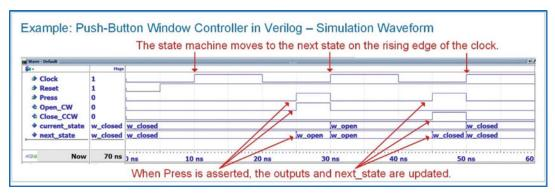
**Example 9.9**Push-button window controller in verilog: simulation waveform
