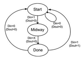
Fig. 7.42 FSM 1 state diagram
