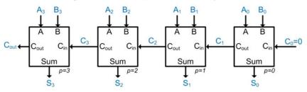
The sum of position 1 cannot complete until it receives the carry in  $(C_1)$  from the sum in position 0. The position 2 sum cannot complete until it receives the carry in  $(C_2)$  from the sum in position 1, etc. In this way, the carry "ripples" through the circuit from right to left. This configuration is known as a Ripple Carry Adder (RCA).
