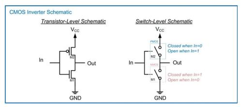
Fig. 3.22 CMOS inverter schematic
