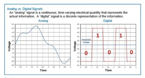
Fig. 1.1 Analog (left) vs. digital (right) signals
