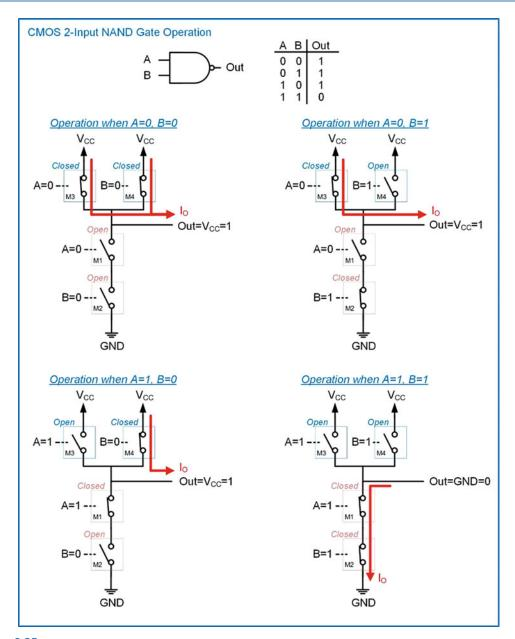
Fig. 3.25 CMOS 2-input NAND gate operation
