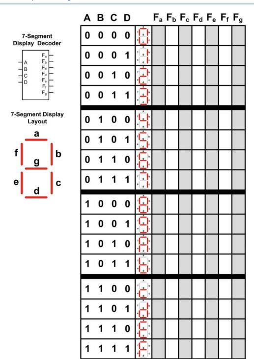
Fig. 6.3 7-segment display decoder truth table
