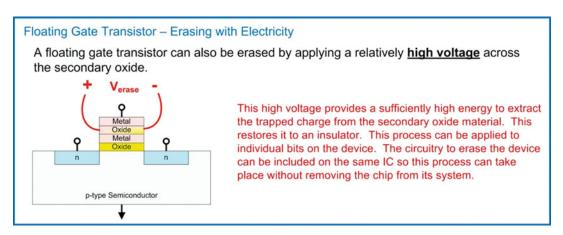
Fig. 10.9 Floating-gate transistor – Erasing with electricity
