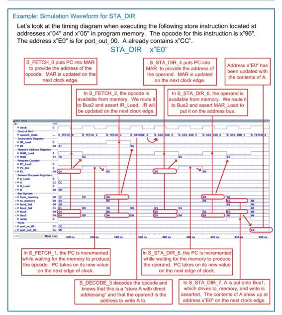
**Example 13.17**Simulation waveform for STA DIR
