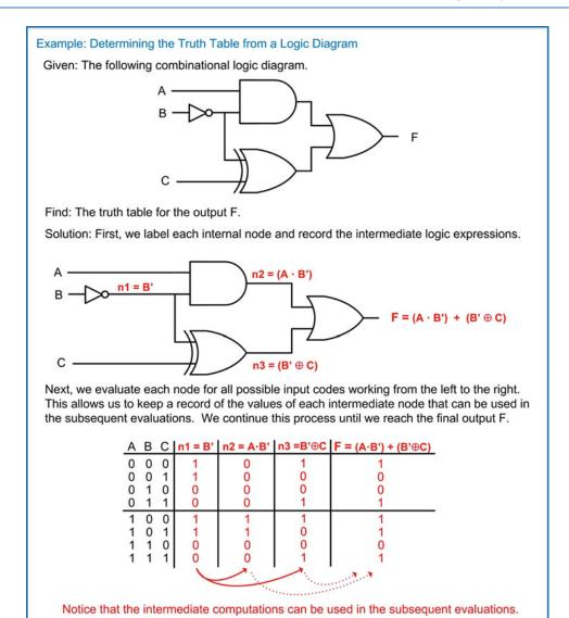
**Example 4.13**Determining the truth table from a logic diagram
