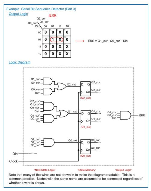
**Example 7.11**Serial bit sequence detector (part 3)
