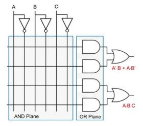
Fig. 11.13 Blank PAL schematic
