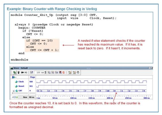
**Example 9.21**Binary counter with range checking in verilog
