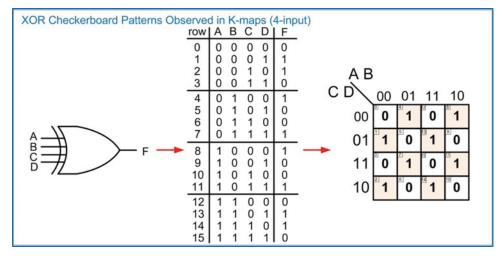
Fig. 4.23 XOR checkerboard pattern observed in K-maps (4-input)
