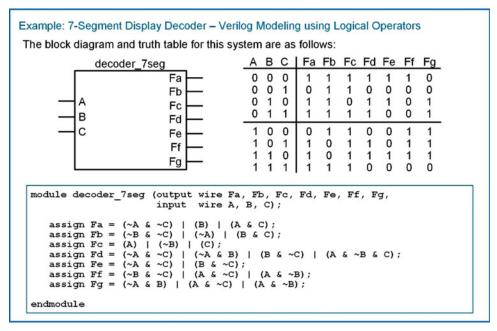
**Example 6.6**7-Segment display decoder: Verilog modeling using logical operators
