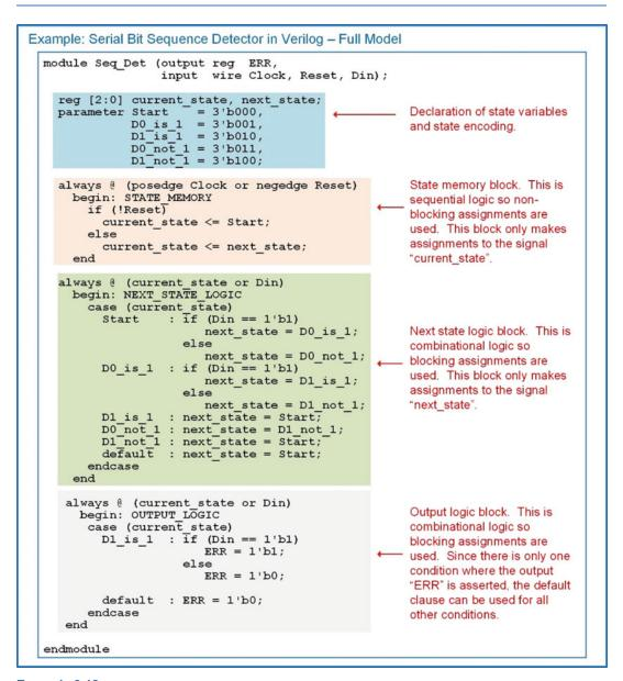
**Example 9.12**Serial bit sequence detector in verilog: full model
