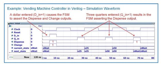
**Example 9.16**Vending machine controller in verilog: simulation waveform
