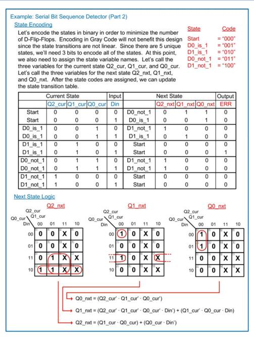
**Example 7.10**Serial bit sequence detector (part 2)
