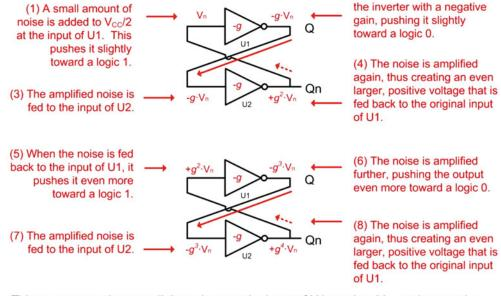
This process continues until the voltage at the input of U1 reaches  $V_{\text{CC}}$  and cannot be increased further. Simultaneously, the voltage at the input to U2 is decreased until it reaches GND and cannot be decreased further. At that point, the system is at a stable state and will store Q=0.
