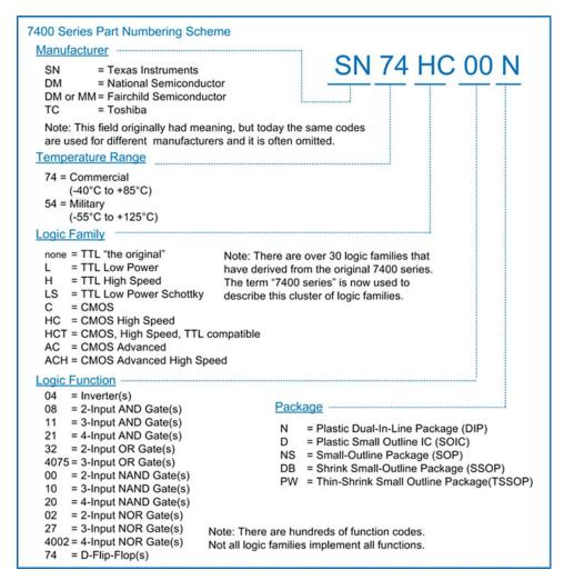
Fig. 3.32 7400 series part-numbering scheme
