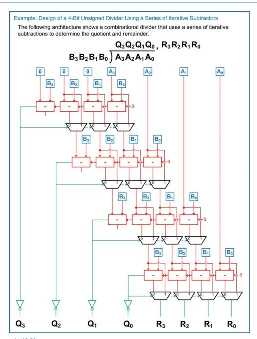
**Example 12.28**Design of a 4-bit unsigned divider using a series of iterative subtractors
