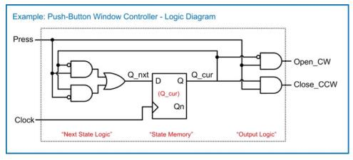
**Example 7.8**Push-button window controller: logic diagram
