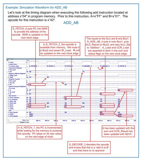
**Example 13.19**Simulation waveform for ADD\_AB
