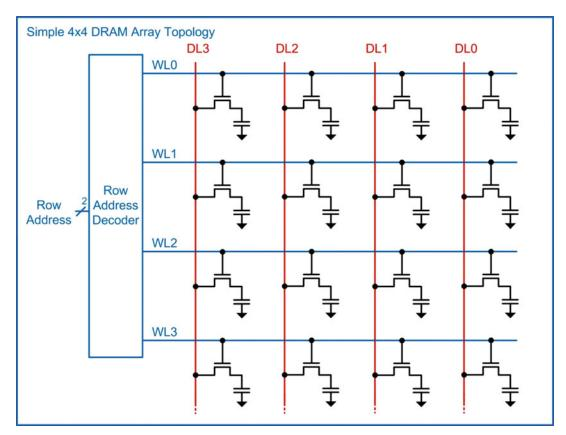
Fig. 10.16 Simple 4×4 DRAM array topology
