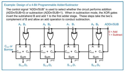
**Example 12.17**Design of a 4-bit programmable adder/subtractor
