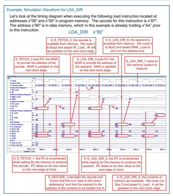
**Example 13.15**Simulation waveform for LDA DIR
