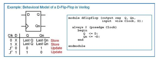
**Example 9.2**Behavioral model of a D-flip-flop in verilog
