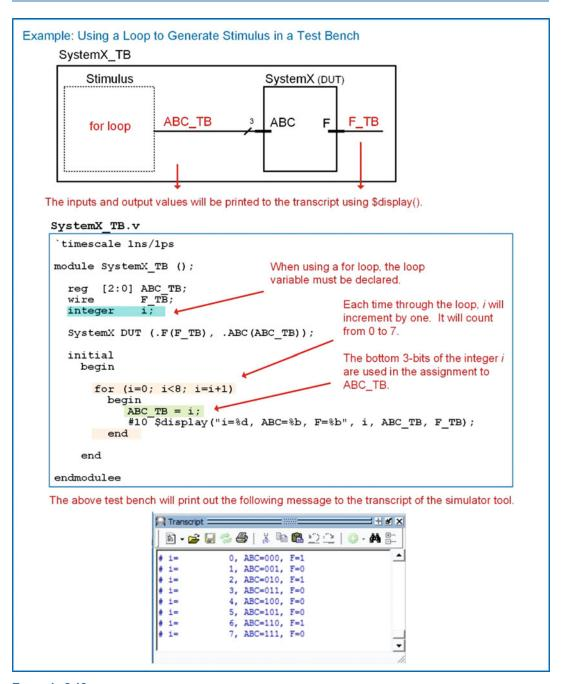
**Example 8.13**Using a loop to generate stimulus in a test bench
