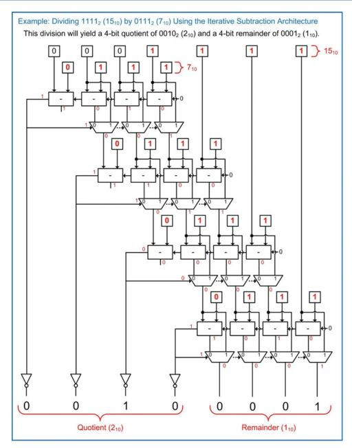
**Example 12.29** Dividing 1111<sub>2</sub> (15<sub>10</sub>) by 0111<sub>2</sub> (7<sub>10</sub>) using the iterative subtraction architecture
