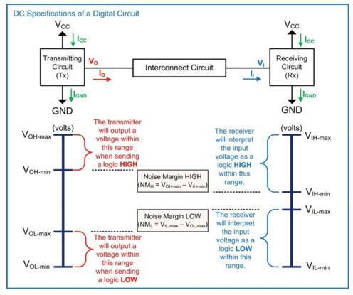
Fig. 3.16 DC specifications of a digital circuit
