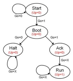
Fig. 7.46 FSM 3 state diagram
