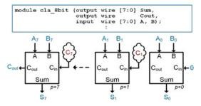
Fig. 12.6 4-bit CLA module definition
