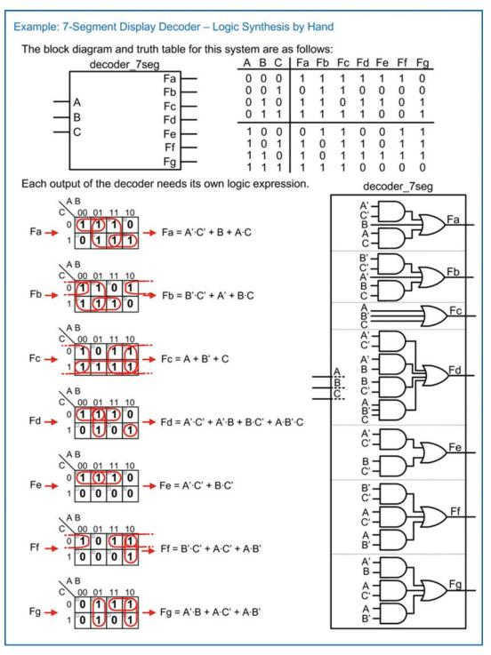
**Example 6.5**7-Segment display decoder: logic synthesis by hand
