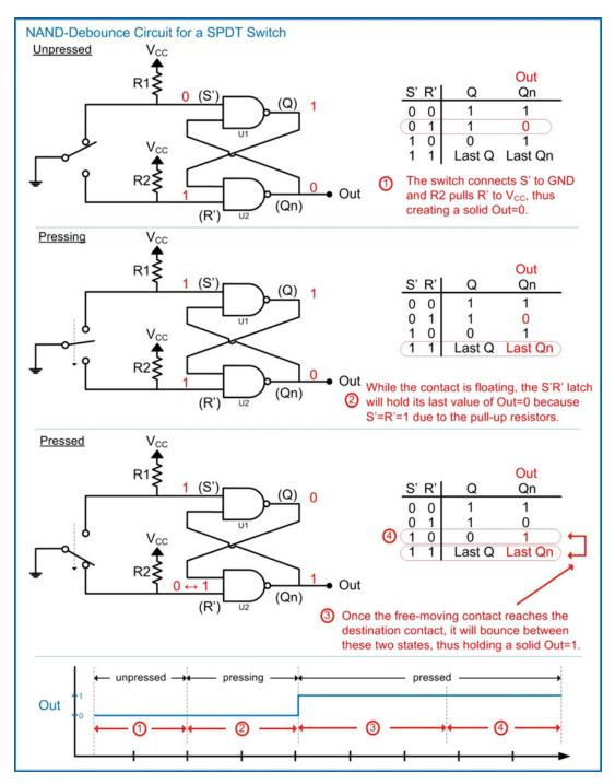
**Fig. 7.27** NAND-debounce circuit for a SPDT switch
