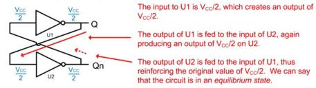
Now let's consider how this circuit responds when a small amount of positive noise  $(V_n)$  is added to the input of U1 when it is at  $V_{CC}/2$ . The  $V_{CC}/2$  component is not shown for simplicity.
