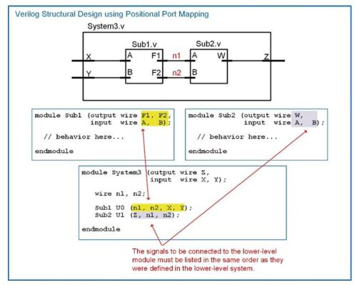
**Example 5.8**Verilog structural design using positional port mapping
