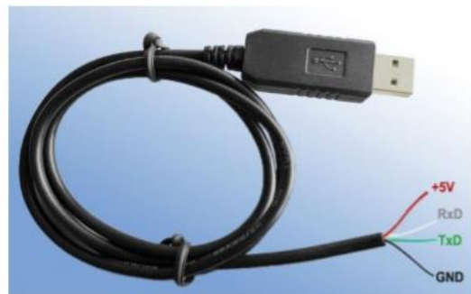
Gambar 3. 4 USB to TTL/ Converter USB UART[21]
