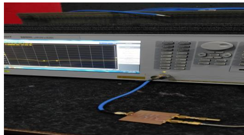
Gambar 3.5 Pengukuran Power Combiner
