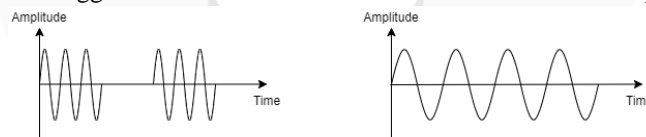
Gambar 2. Output sinyal pulse wave radar dan continuous wave radar
