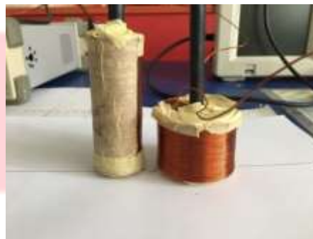
Gambar 3 Koil Transmitter dan koil Receiver
