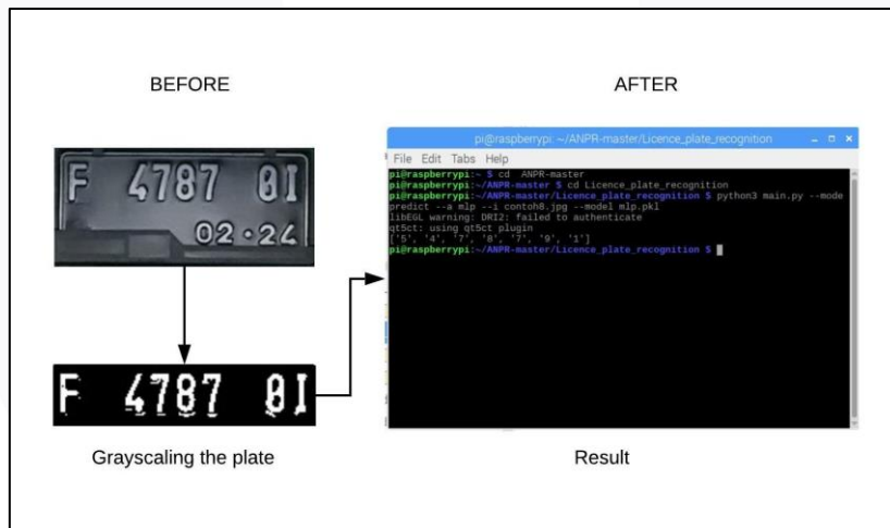
Figure 3.3 Real time Object detection result.
