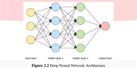
As explained in Figure 2.2 Deep Neural Network architecture is a multilayers process. The above architecture is commonly referred to as Multilayer Perceptron (MLP) or Fully-Connected Layer[7]. The first architecture has 3 neurons in the Input Layer and 1 Output Layer nodes. Between Input and Output, there is 1 Hidden Layer with 4 neurons. The number of layers depends on the input data. The more input data, the more hidden layers.
