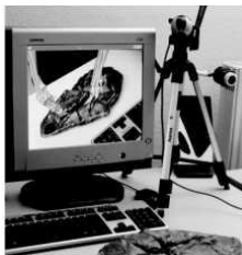
Gambar 3.1.2.1-7 Screen-Based Video See-Through Displays Sumber: Bimber O and Raskar R (2005)
