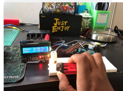
Gambar 4. 3 Sensor DHT22 Membaca Suhu Panas
